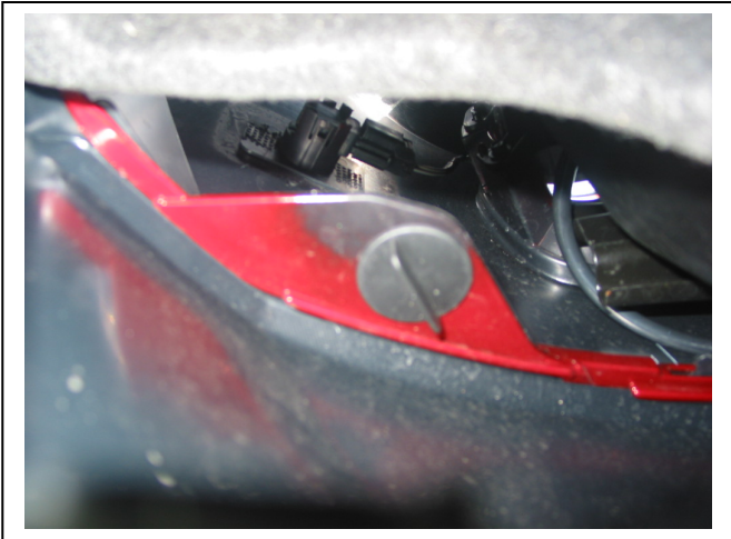
Figure 1: Twist clip holding lower bumper to upper bumper sections
