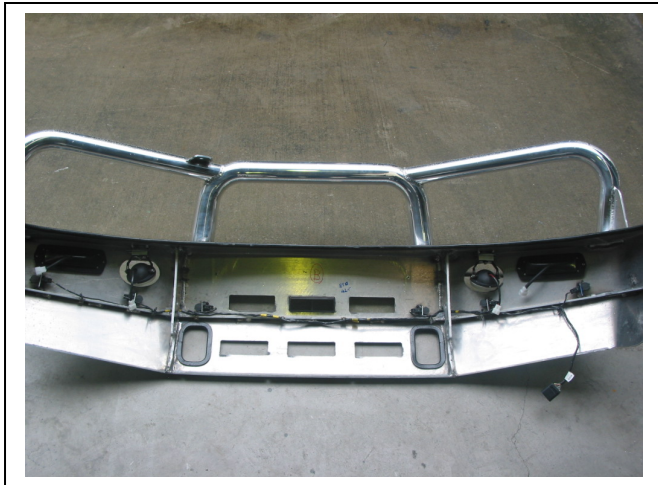
Figure 19: wiring harness wired into rear of Protection bar
