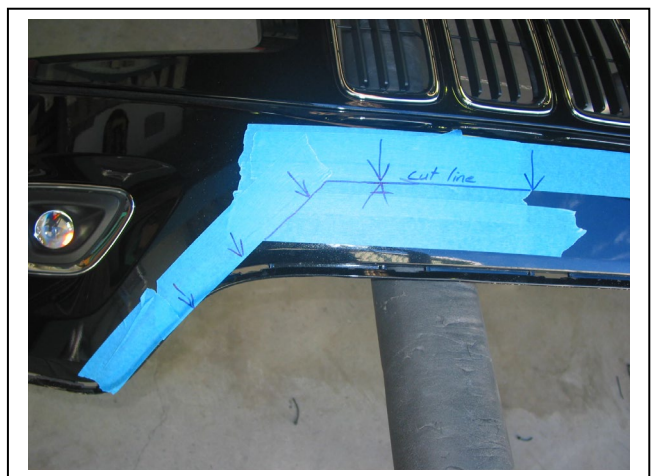
Figure 12: side tape line on bumper. NOTE: Cut line on tape is to the inside.
