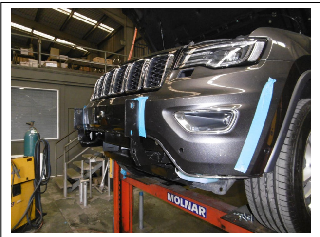
Figure 3: Bumper with lower section fully removed.
