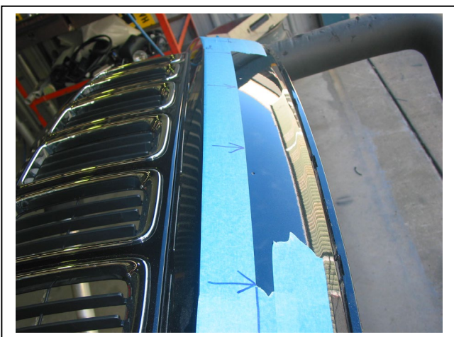
Figure 11: Top tape line on bumper. NOTE: Cut line is to bottom of tape.
