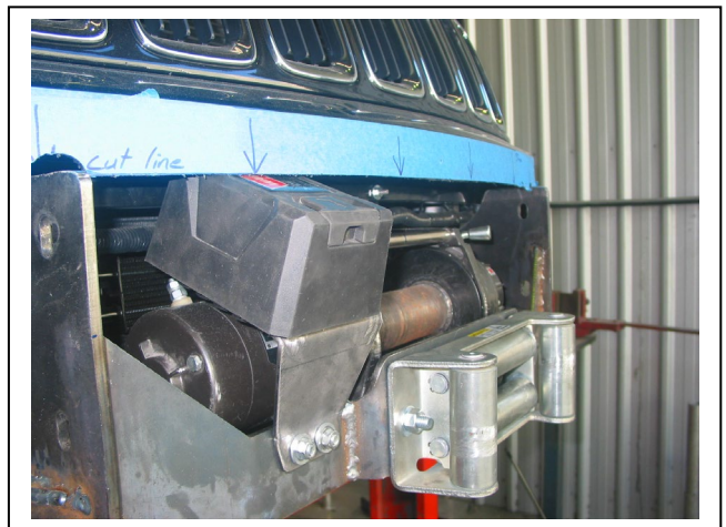
Figure 10: Warn control box mounted to winch frame.
